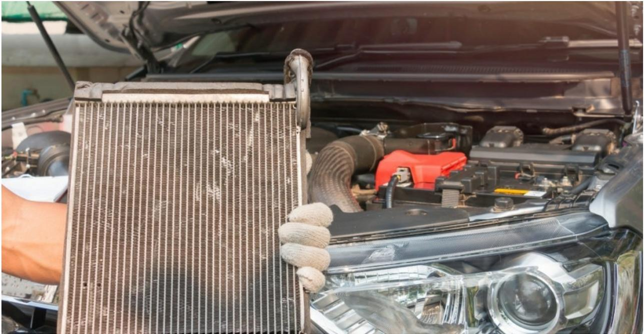
Your car's radiator plays a very important role in keeping your car in driving condition. While you may not notice it immediately, ***a broken radiator, either as a result of a leak or other mechanical issues, can cause serious damage to your engine.***
