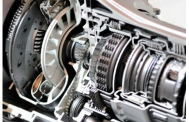
**Transmission** – In order for you to drive your vehicle at a certain speed, the wheels have to have power. ***This is the job of the transmission, which shifts gears and supplies the power to the wheels.*** In a manual transmission vehicle, the engine and transmission are disconnected when you push in the clutch to change gears. In an automatic transmission vehicle, the transmission shifts gears for you.
