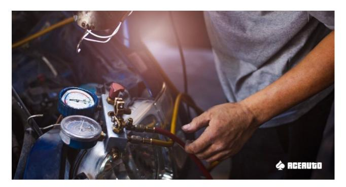
Your <u>car AC compressor</u> is designed to pressurize the refrigerant that is running through the air conditioner. That's what makes your car's AC system produce cool air. To keep the refrigerant flowing through the AC system, and keep it under pressure, and at a high temperature, the AC compressor must work properly. But, naturally, AC compressors eventually need repair or replacement. Here we'll look at the most common symptoms of a broken AC compressor.
